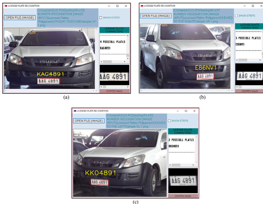
Fig. 12. License Plate Recognition, a) Upright Position; b) Skewed to Right Position; c) Skewed to Left Position
